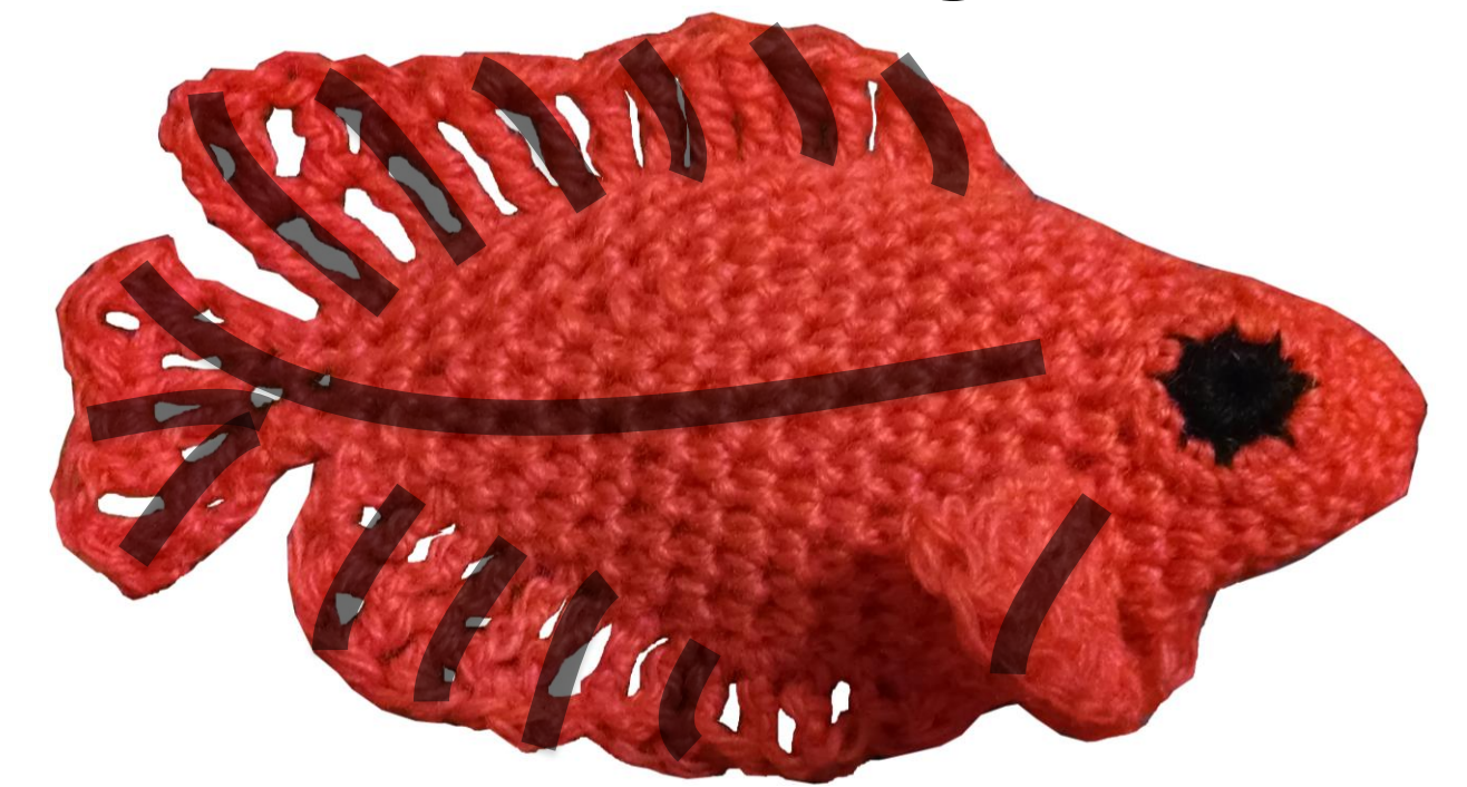
Mock-up of a soft fish with actuator stripes
