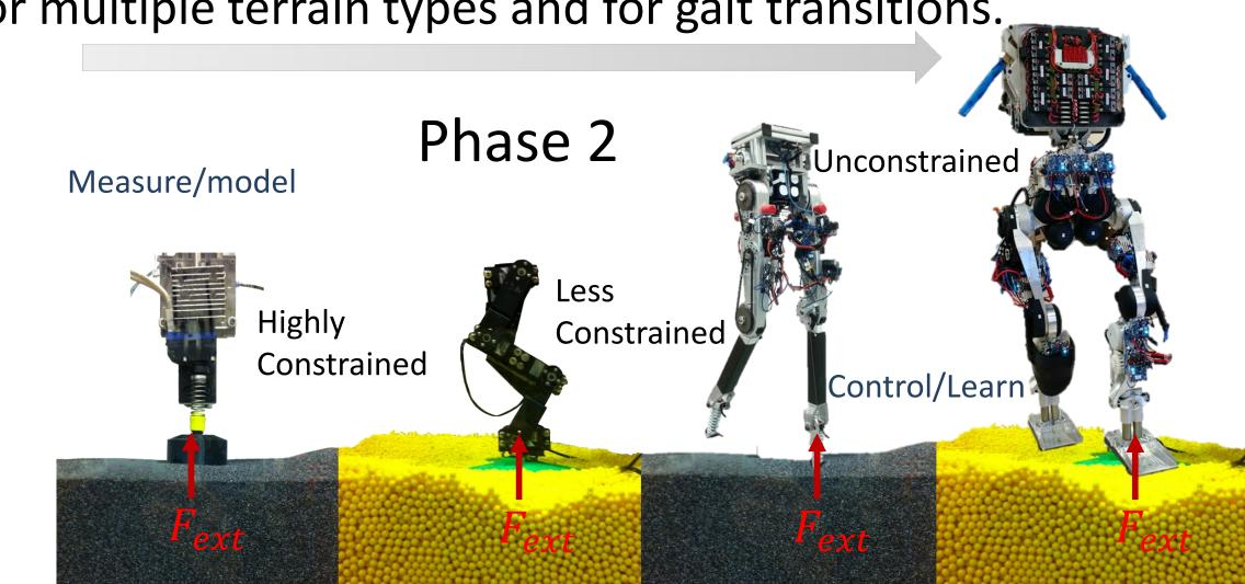
Task 1: Experimentally derive granular force laws for modeling  $F_{ext}$  through Task 3: Learn terrain models controlled experiments.
