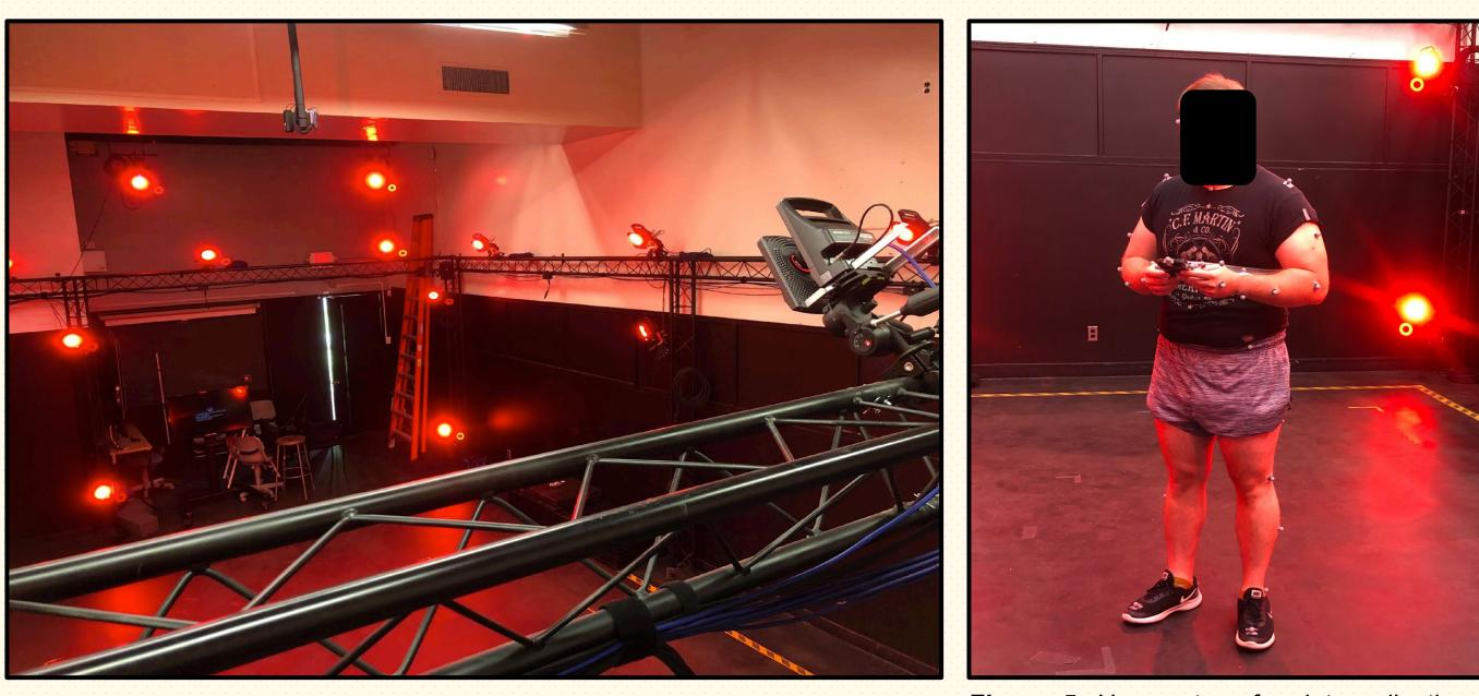
Figure 3. The Motion Capture Studio, as seen from the ground floor. The bright red lights are the IR illumination LEDs mounted on the Vicon cameras.
