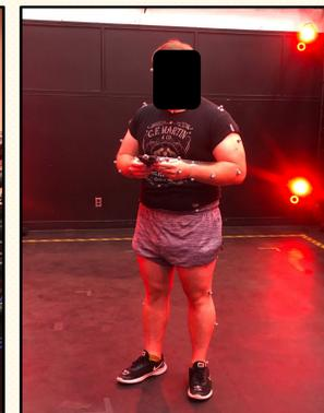
Figure 5. User set-up for data collection. The silver spheres taped to the subject are the sensors monitored by the cameras.
