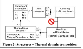
The composed DSML allow-s integrated modeling of Structures and Thermal domains of a component. However, notice that the integrated DSML contains a constraint – a well-formedness rule (stop-sign symbol in Fig) - with the restriction that for every Coupling between two Components, there is a corresponding *HeatFlow*. Models that do not satisfy this constraint are rejected by the GME modeling tool.
