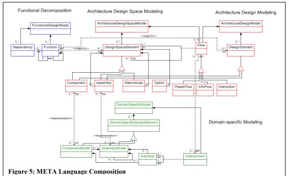
the organization of the domain-specific models (which are stored in third-party, domain specific tools) – these are concrete models using components and assemblies, interconnected
