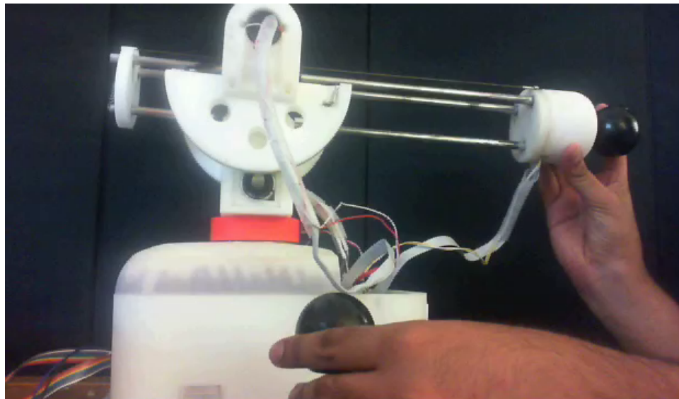
Force-Feedback Interface (5 DoF, developed in-house)
