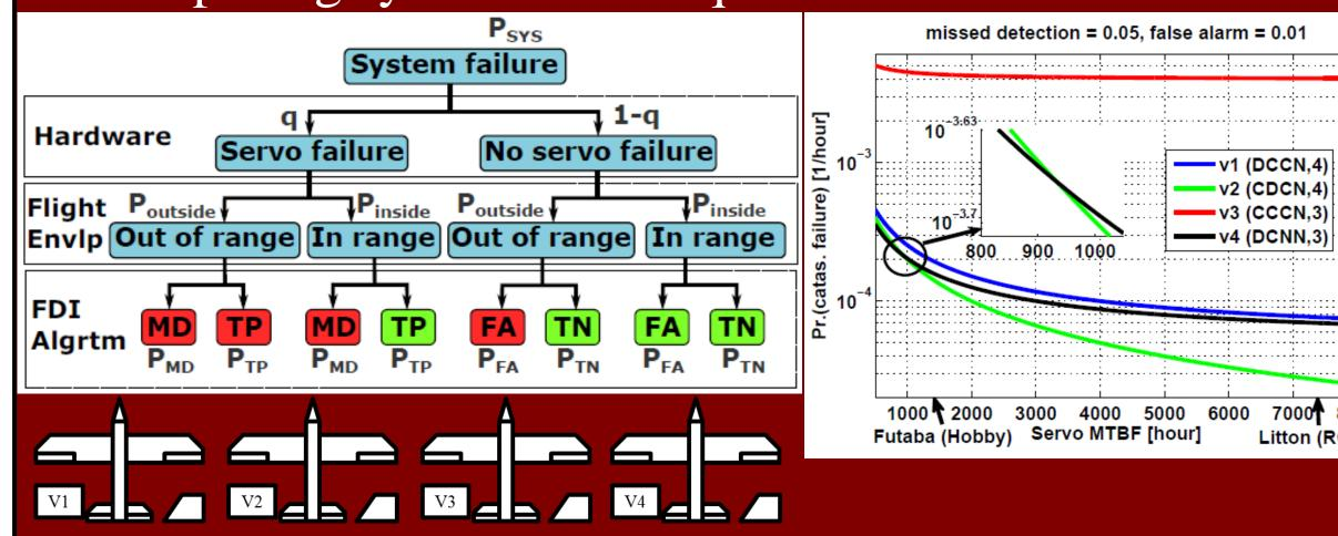
Density-based fault trees are used to assess the reliability of actuator architectures for unmanned aircraft. Task 1.B - Investigate techniques for computing bounds on the probabilistic performance of a system.
