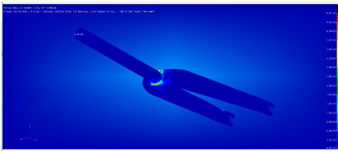
FEA model created programmatically and Tsai-Wu failure criteria computed.
