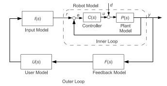
Fig. 1. Block diagram showing the elements in a teleoperation control loop, represented here as transfer functions. The robot's processes (including all levels of autonomy, if present) run in the inner loop, while the operator provides the control for the outer loop.
