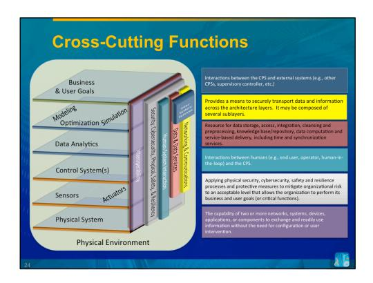
• The cross-cutting functions are the means and methods to securely and reliably transport data and information across the architecture layers.
