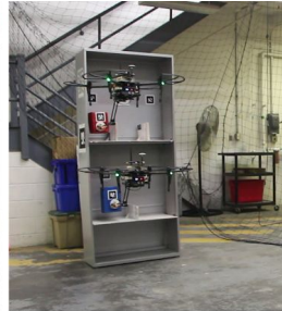
JHU AirGripper performing package sorting
