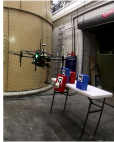
JHU AirGripper performing package sorting
