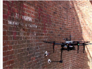
environmental sensor placement
