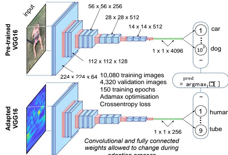
Pretrained VGG16 structure and transfer for EEG-based action prediction
