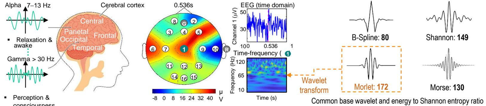
Brain structure and wavelet transform of brainwaves into time-frequency images
