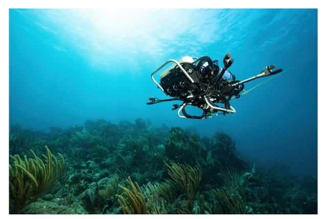
Developed CUREE: a novel robot for visually and acoustically guided missions in coral reef like environments
