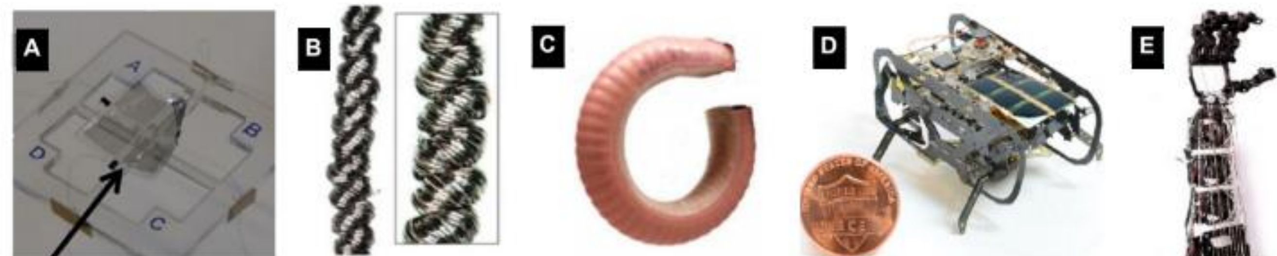
Figure 1: (a). Dielectric elastomer actuator [2]. (b). Supercoiled polymer actuator [3]. (c). Soft fluidic actuator [4]. (d). A hexapod robot driven by piezoelectric actuators [5]. (e). A robot hand driven by SCP actuators [3].
