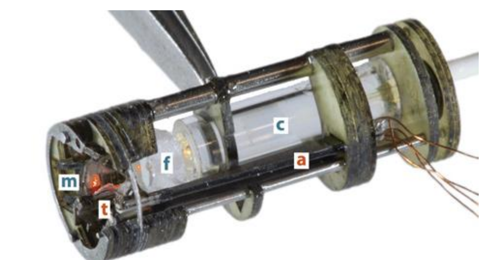
Figure 7: Example outcome of high performance artificial muscles: the creation of a piezoelectric laser-steering compact (6mm diameter) surgical tool.
