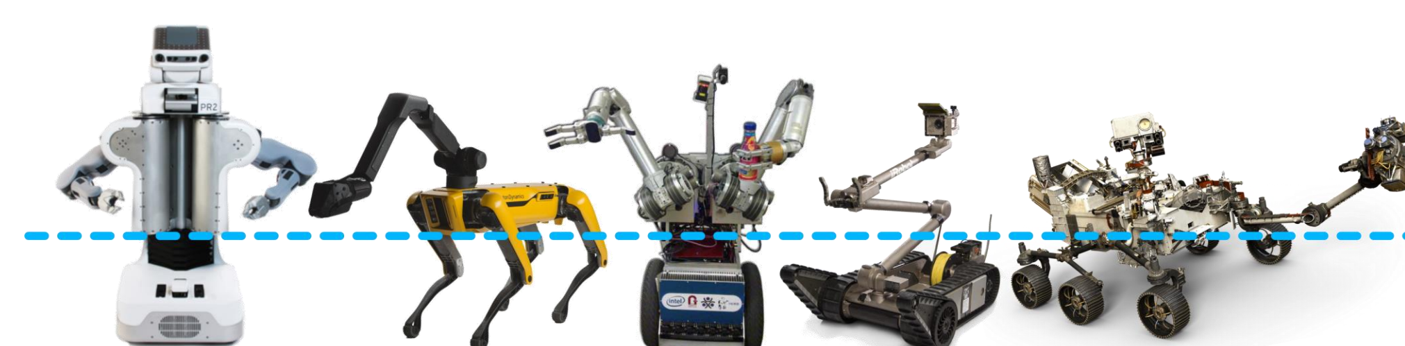
Most mobile manipulation systems are built by combining independent manipulation and locomotion system.
