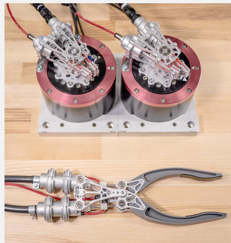
2-DOF gripper, driven by remote direct-drive brushless motors
