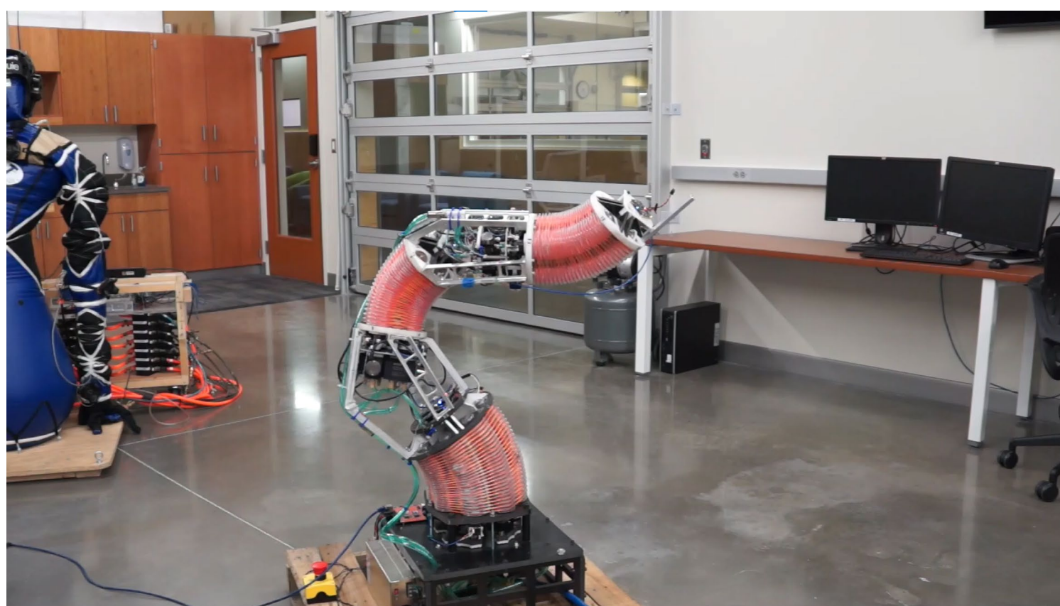
Past research in our group, on learned or adaptive soft robot control for large-scale manipulators, shows that soft robots are a viable option for human-robot co-manipulation.
