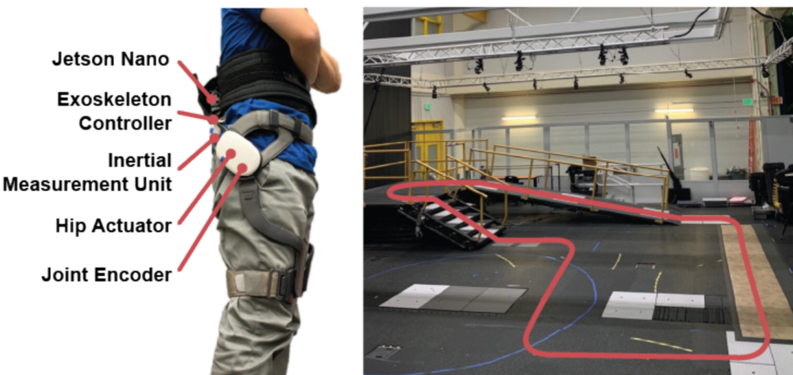
Experimental Setup for Controlling Human Subject Gait Phase Estimation Data
