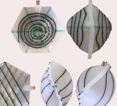
The PneuSMA actuator is controlled via activation of different SMA springs within the actuator, in conjunction with pneumatic actuation. The actuator demonstrates remarkable spatial controllability evidenced by testing under different pressures and SMA activation combinations.
