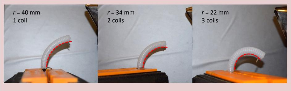
Combined pressurization of the cavity and contraction of the SMA coils results in an apparent increase in stiffness of the actuator.
