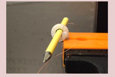
Here we relate the tendon forces to the resulting configuration of the element in static equilibrium for any set of axes selected (melted). In this relationship, we model the melted axes as torsional springs with constant stiffness to represent the elastomer's resistance to bending.
