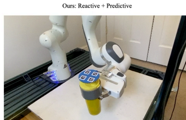
Robot slows down to pick up object and then speeds up to reach goal location
