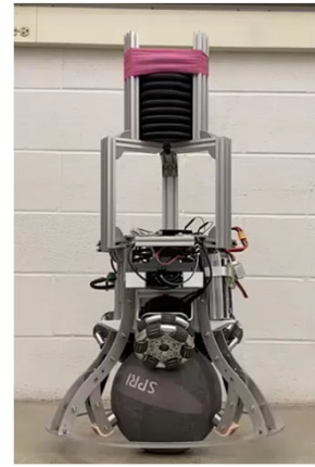
Self balancing w/ 50 lb load
