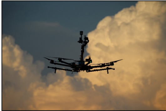
M600 with gimbal mounted Ultra-Sonic Anemometer
