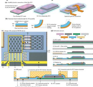
**Achievement:** Fabrication approach integrates thin-film PZT materials with electro-thermal micro-origami systems to enable sensing, precise actuation, and control. (Ref. 1)
