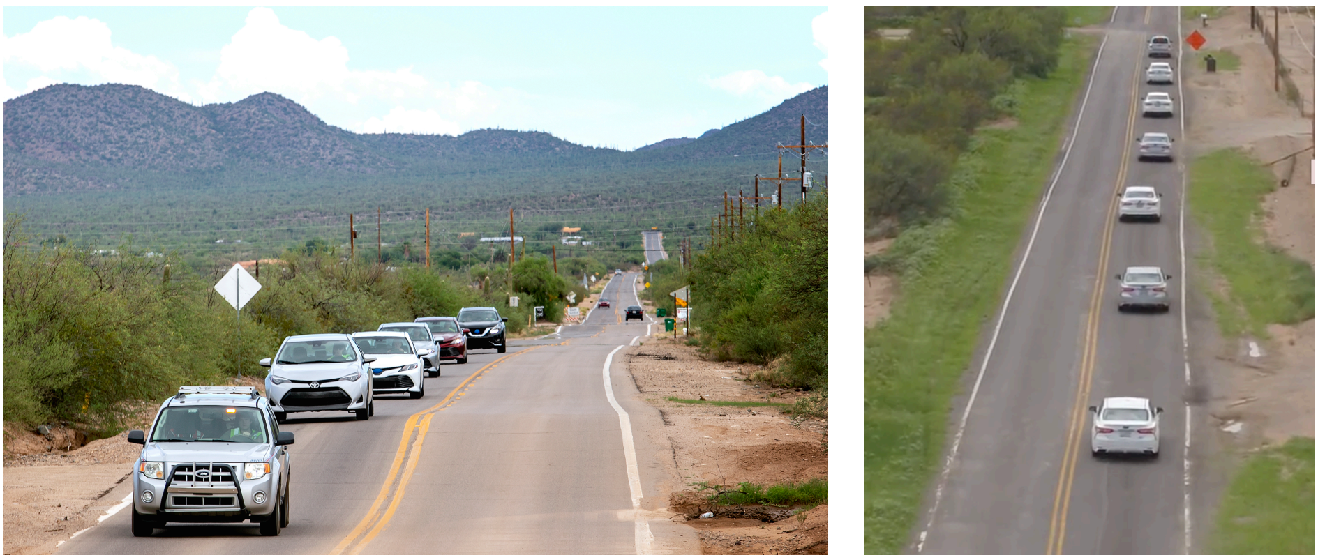
Platoons of vehicles were driven in a series of testing events, taking place in Tucson AZ, in order to record stability of ACC vehicles.
