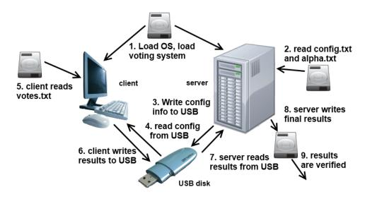
EVS consists of a server (election management system) and client (voting station) with sneakernet USB for data transfer
