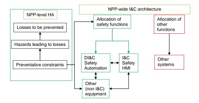
Figure 6: NPP-wide I&C architecture—allocation of functions in the concept phase.
