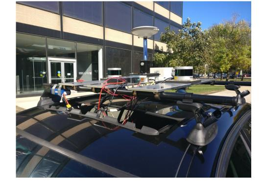
GPS, IMU, and lidar experimental setup (top) and example lidar point cloud with features extracted (bottom)
