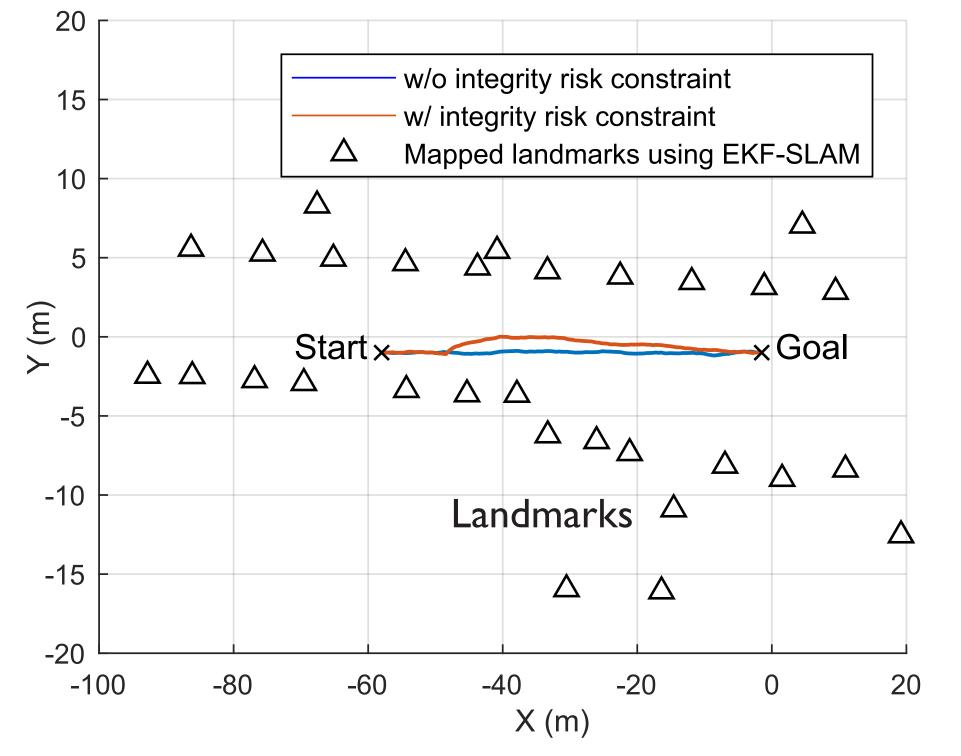
Integrity-risk constrained model predictive control (MPC) shows how a robot will decrease its integrity risk by moving away from landmarks that are ill-separated
