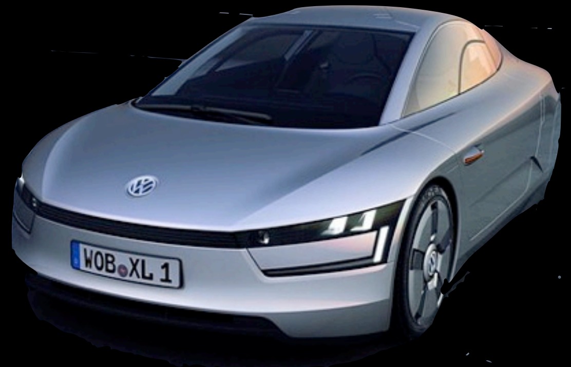
VW XL1 2-seat plug-in hybrid (2011), 1,752 lb, 230 mpg gasoline , 2013 production
