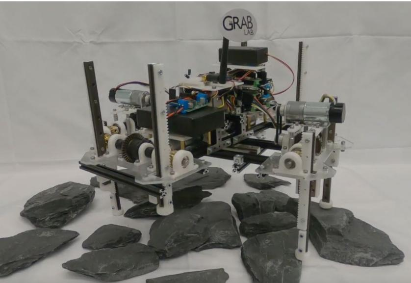
Developed a full-mobility legged robot with passively adaptive legs In favor of compact design and controllability, legs also perform pitch/roll motions Bidirectional leg actuation improves stability on compliant terrains Stable locomotion demonstrated in unterhered outdoor testing
