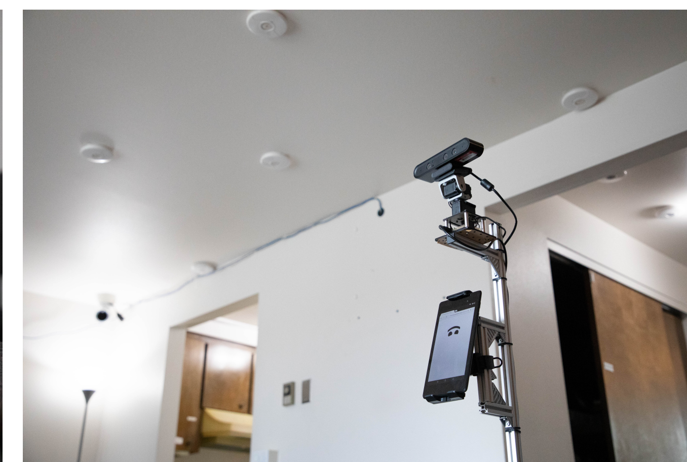
Fig. 6. Passive infrared motion sensors are installed on ceilings of the smart homes.
