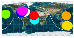
Figure 2: This orbit ground track shows several ground station locations and their ranges. At some locations, the satellite sees several ground stations, whereas, at other locations, the satellite is just barely out of range. Robust capacity-constrained scheduling is aimed at optimizing the transfer of data from space to ground.
