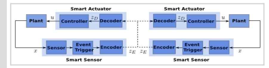
• Shared communication channels with possibly low, time-varying, unreliable capacity • Induced communication delays and finite precision (quantized) feedback
