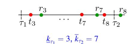
• Equivalent to optimal allocation of *discrete* # bits to be transmitted in each time slot
