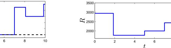
$R(t) = R_j, \quad \forall t \in (\theta_j, \theta_{j+1}], \quad \text{min comm. rate: } \frac{p_k}{\Delta(t_k, p_k)} \ge R(t_k)$  $\bar{p}(t) = \bar{\pi}_{j}, \ \forall t \in (\theta_{j}, \theta_{j+1}], \ \text{max packet size: } p_{k} \leq \bar{p}(t_{k})$ • Channel is not available when  $\bar{p} = 0$  (*channel blackout*) • Channel evolution is known a priori
