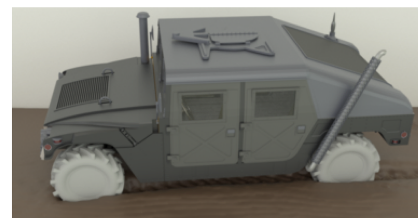
Preliminary results: Rendering of a vehicle driving on mud simulated using hybrid MPM.
