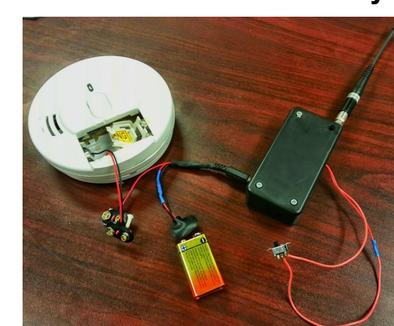
Hacked 9-volt smoke sensor sends alerts over Sigfox UNB (Arduino-powered)
