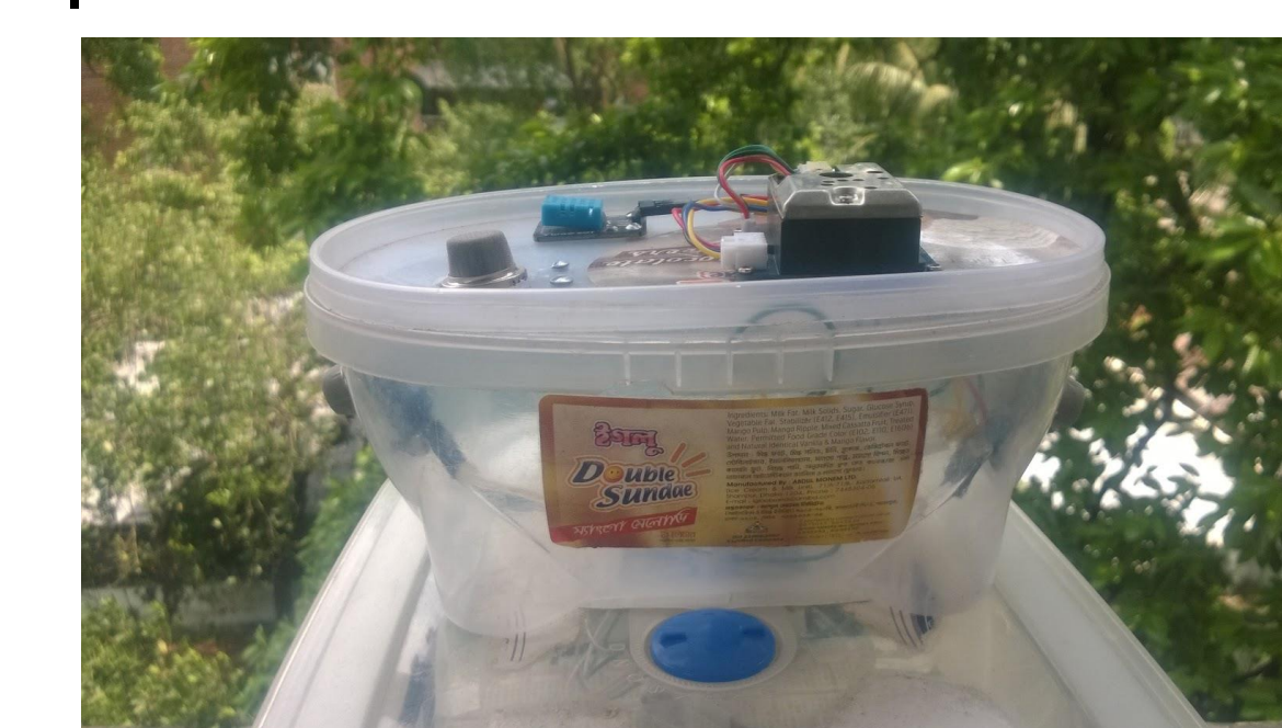
EnviroSCALE box deployed in Bangladesh with 3G modem and multiple types of gas sensors to monitor air quality
