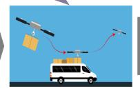
The proposed delivery network is comprised of autonomous flying robots and existing transport networks (public and private ground vehicles).
