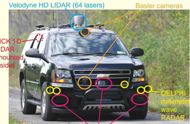
Ibeo LIDAR scanners (4 lasers)
