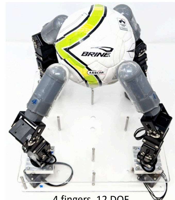
4 fingers, 12 DOF Tactile sensors (distal only) No torque sensing
