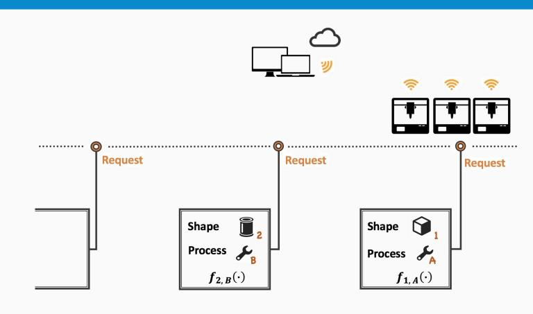
A significant trajectory of additive manufacturing (AM) technologies is cyber-physical AM systems (CPAMS) that seamlessly integrate computer-aided design models and physical AM processes.
