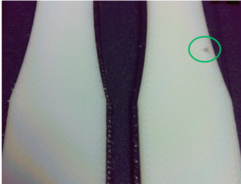
Build paused halfway to show void
