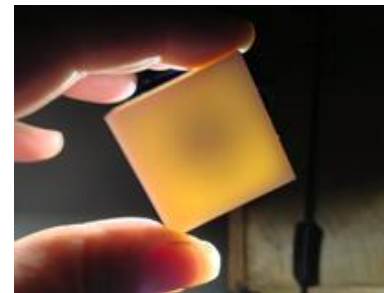
Functioning Embedded RFID tag (horizontal cavity)
