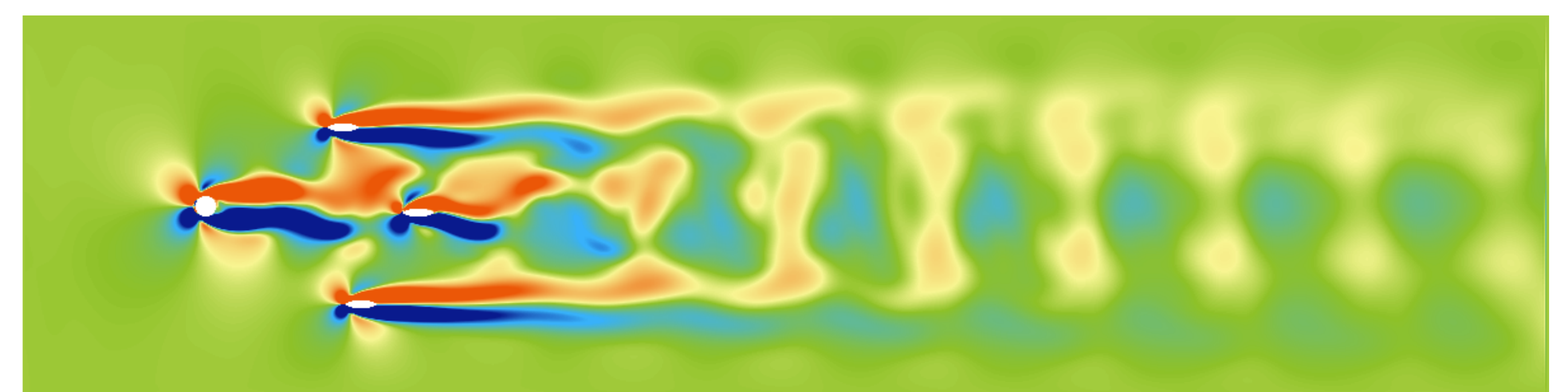
Figure 2. the WebGL 2.0 implementation of the LBM method provides an interactive simulation of the flow around obstacles that can be added interactively during simulation. For more information on these simulations see reference [2].
