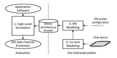
Pre-characterized EM macro-models are composable, allowing on-the-fly prediction of EM fields for application software.
