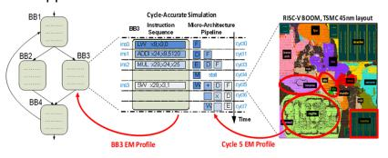
Hierarchical macromodeling: Software is compiled into basic blocks (BBs) of instruction sequences. Spatio-temporal component-level EM profiles are composed into cycle-by-cycle and block-by-block profiles of software executing on the processor.
