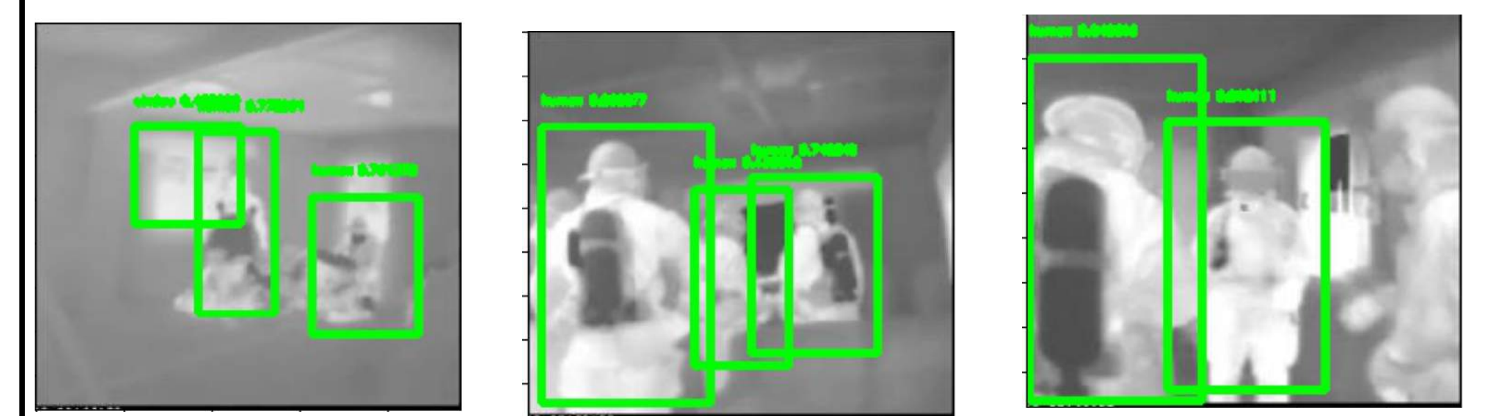
Figure 5. Demonstration of object detection and tracking implemented with Faster RCNN. The green boxes bind the object of interest. The label on top infers corresponding object and detection probability. Selected objects of interest include firefighters and civilians, doors, windows, and ladders.
