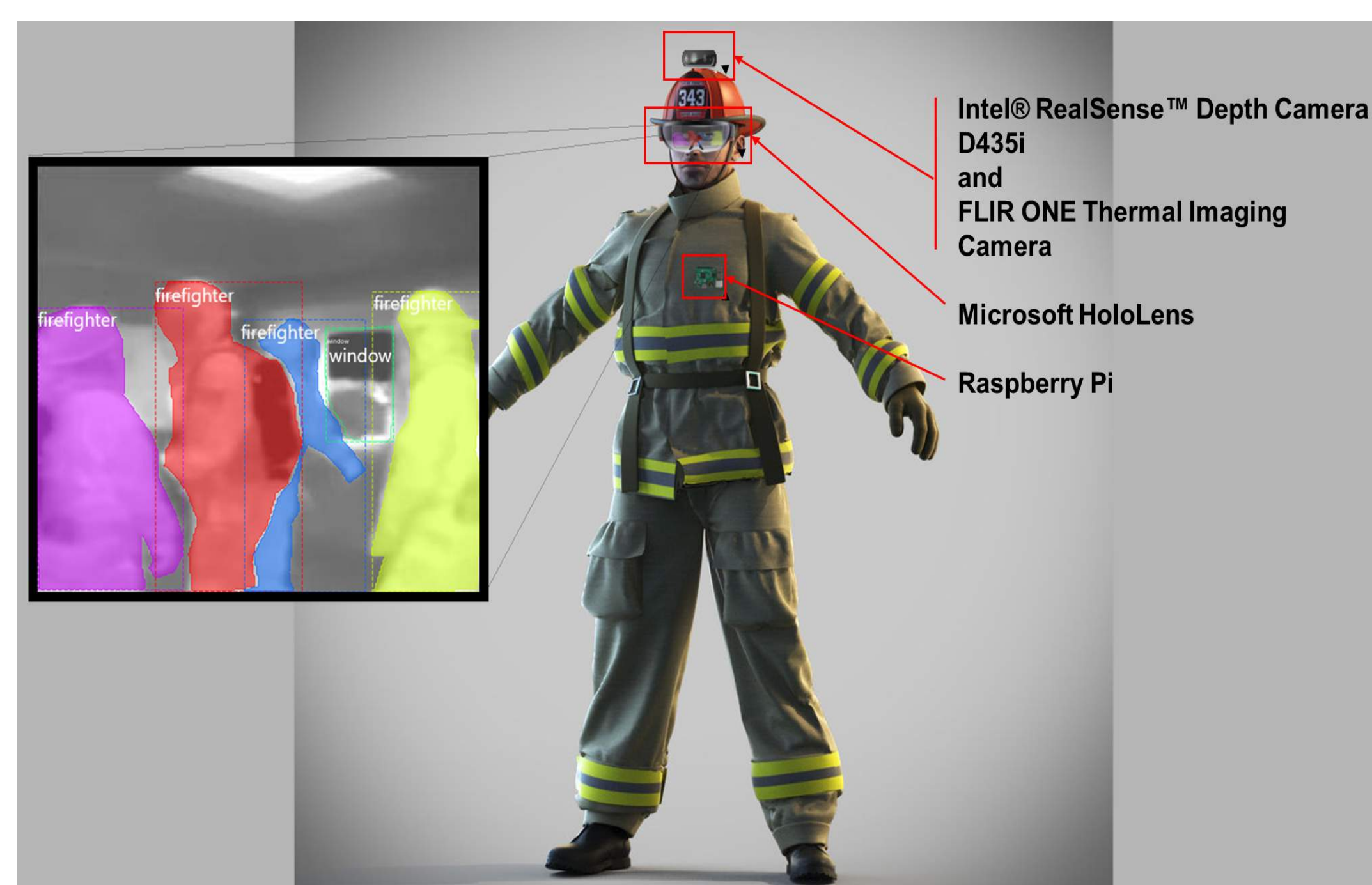
Figure 4. Illustration of System Deployed as Part of a Firefighter's Gear. The embedded system is demonstrated as part of the firefighter's integrated gear.
