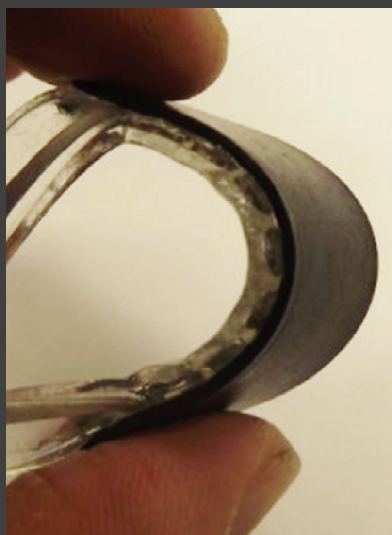
Rigidity tuning element with shape memory polymer (Wanliang Shan & Carmel Majidi)
