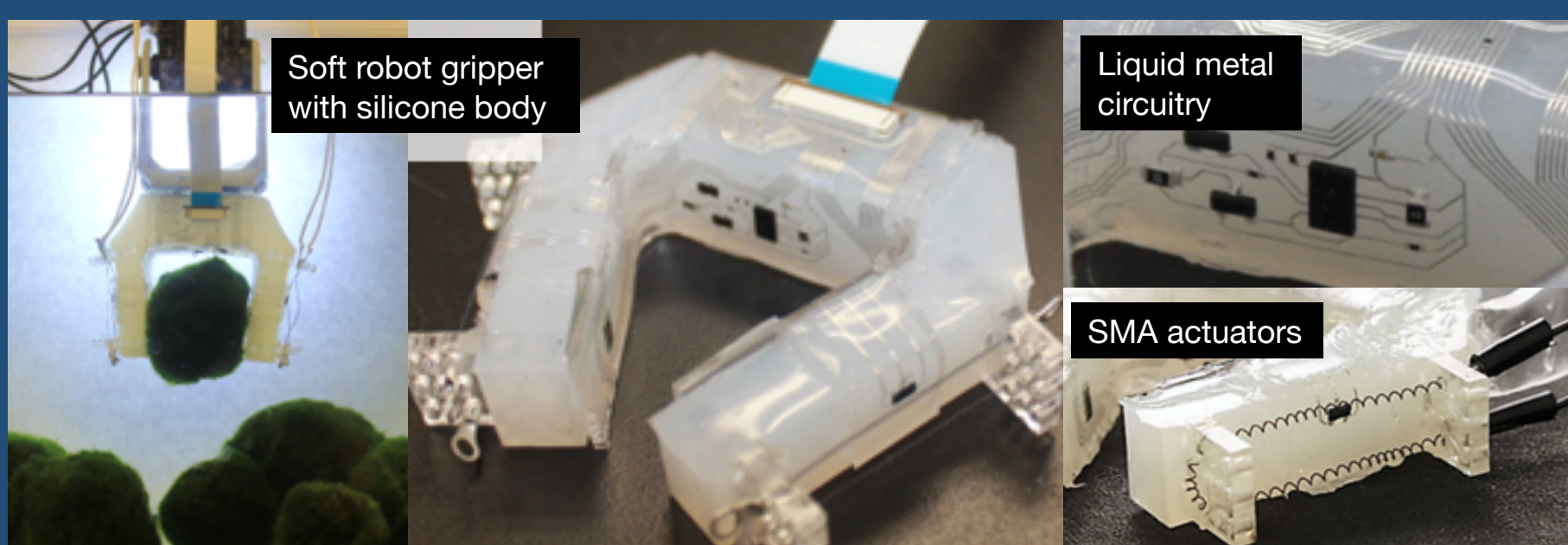
Soft electronic skin using liquid metal circuitry (Carmel Majidi)
