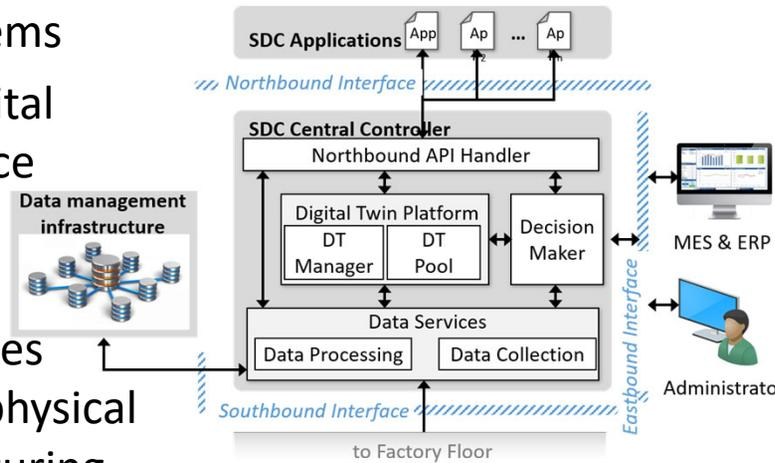
**Software-Defined Control, flexible control reconfiguration to enhance performance**
