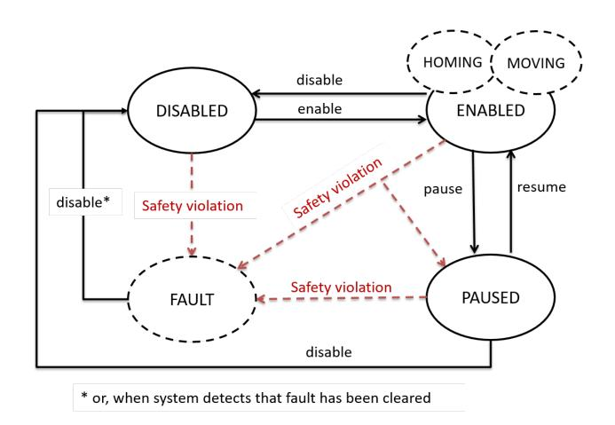
Meta-state queries: is\_disabled, is\_enabled, is\_paused, is\_fault Operating mode queries: is\_homing, is\_moving, is\_homed
