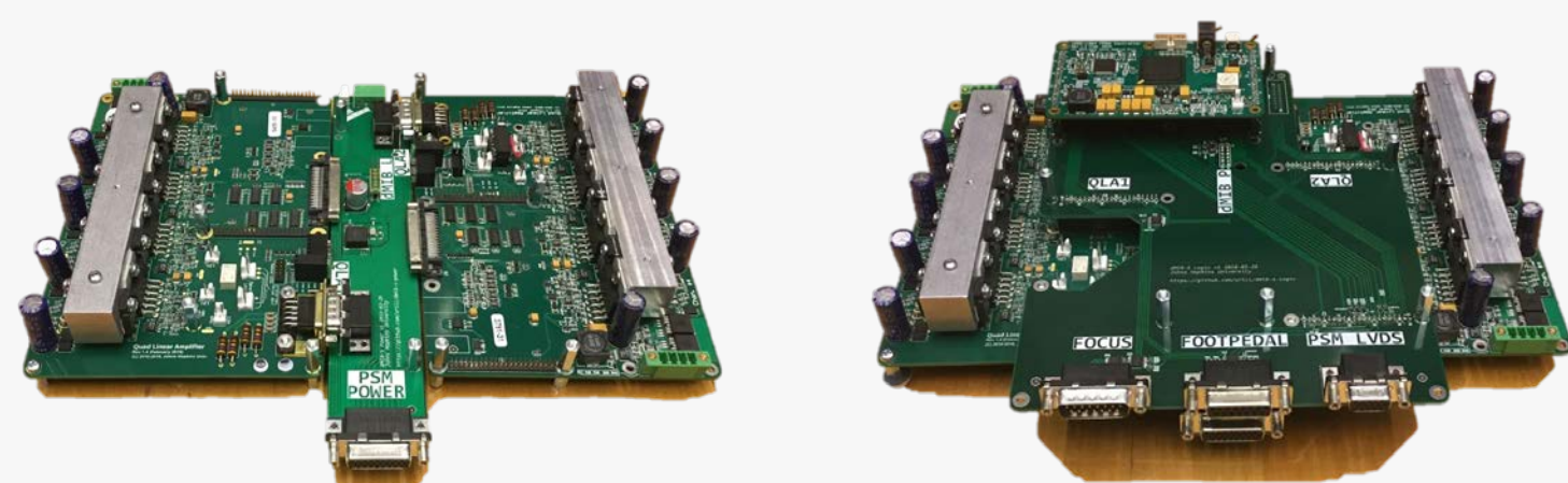
da Vinci S controller (2xQLA + FPGA + custom boards)
