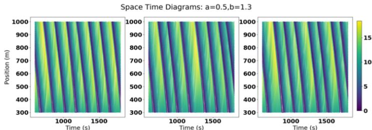
**FIGURE 4** : Three time space diagrams colored by speed in (m/s) produced from identical simulations except for the random seed, with  $(a, b) = (0.5, 1.3)$ . Waves are present and small variations occur in the phase and amplitude of the waves.
