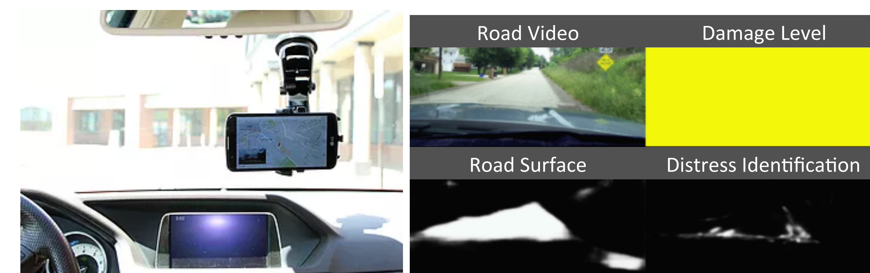
Automated Road Surface Condition Assessment from smartphone captured images and AI methods. Formed company RoadBotics to collect road data and perform analysis. Results provided to clients (e.g., all levels of government, planning organizations, and engineering/construction firms) as easy-to-ready color-coded maps on a web-based platform.
