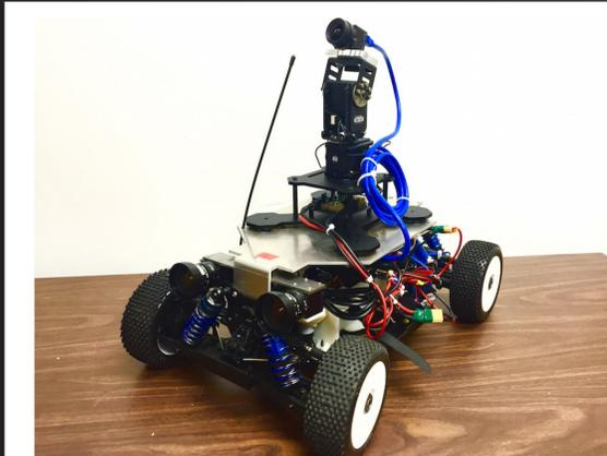
The Ninja Car is a  $\frac{1}{8}$ -scale model of a car that has been modified for autonomous operation using **on-board sensing and computation**. The API for the vehicle’s control and sensing algorithms provide the inputs available for many levels of controller synthesis.
