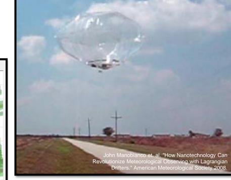
Ground-released LD have successfully been used to measure the forward flank downdraft<sup>1</sup>.
