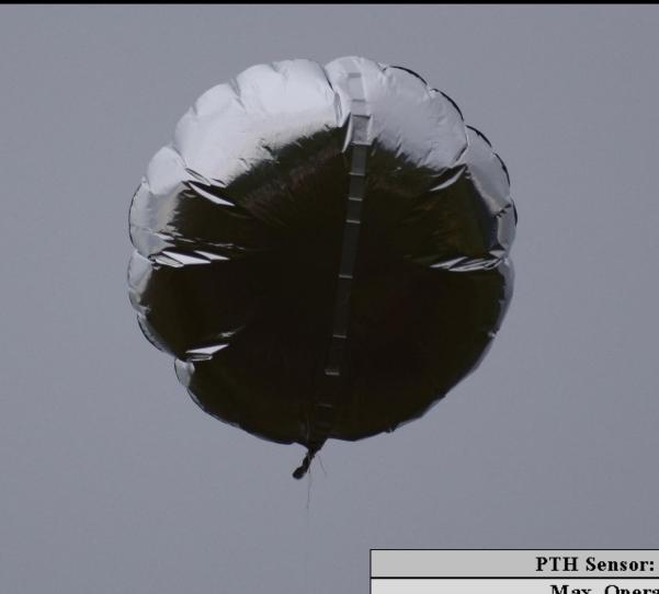
Drifter He Capacity: 125L Can lift a payload of 92.5g to 10,000 ft.
