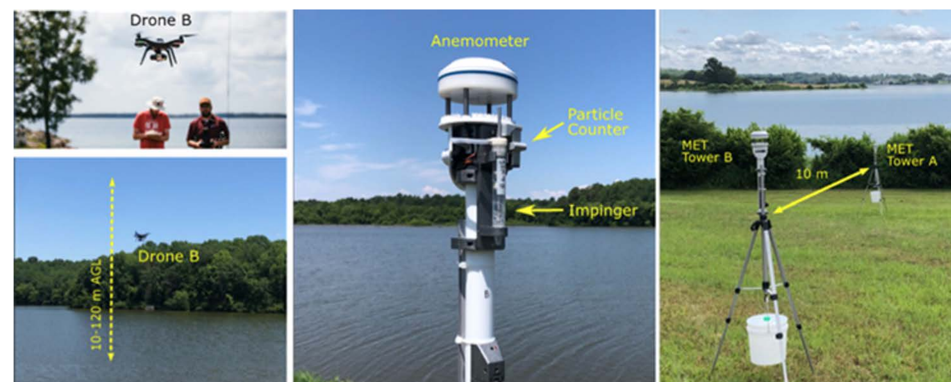
Figure 2. Drone-based wind velocity profiles were measured from 10 to 120 m above ground level. Concurrent meteorological data was collected on board a pair of Stationary Impinger and Sonic Anemometer Tripods (SISATs) placed near the shore of Lake Anna.
