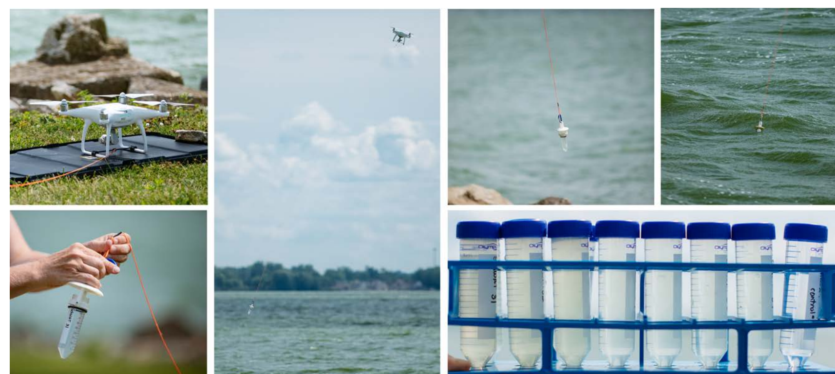
Figure 1. Water was sampled using a drone-water sampling system. This consisted of 3D-printed sampling device tethered to a drone, and was used to collect surface water samples from the shore along transects of 100 meters.
